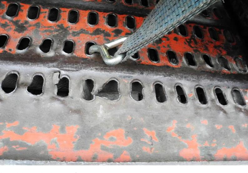
Regularly inspect the check plate for wear and tear.
