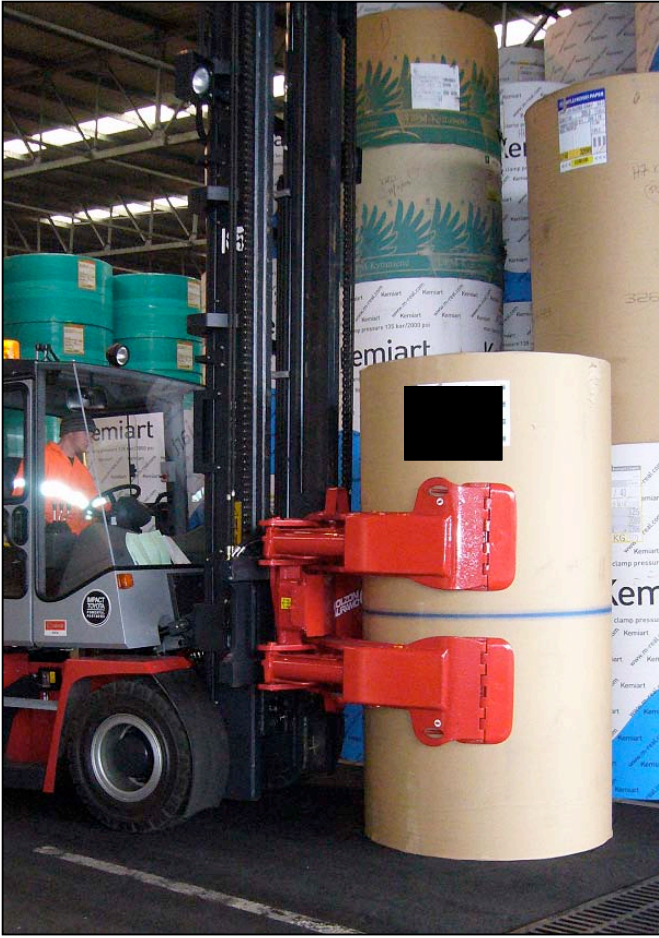
The type of clamp truck used in the loading operation is shown in the photograph to the left.
