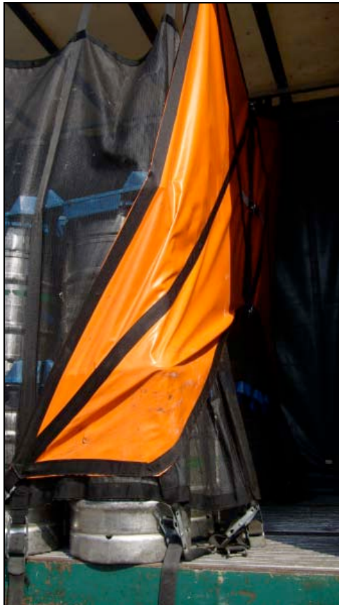
The inner curtain was secured to a rail running the length of the trailer. Again, the “sail” was used to provide rear containment
