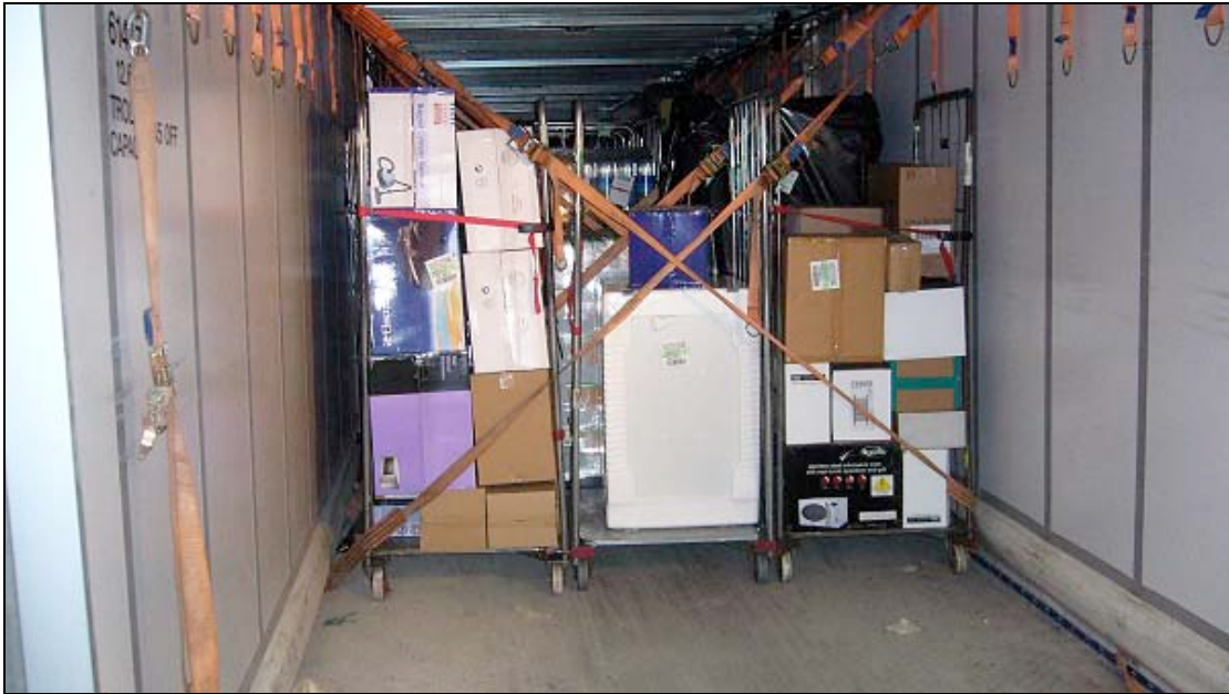
Cross-strapping on Company 7 trailers
