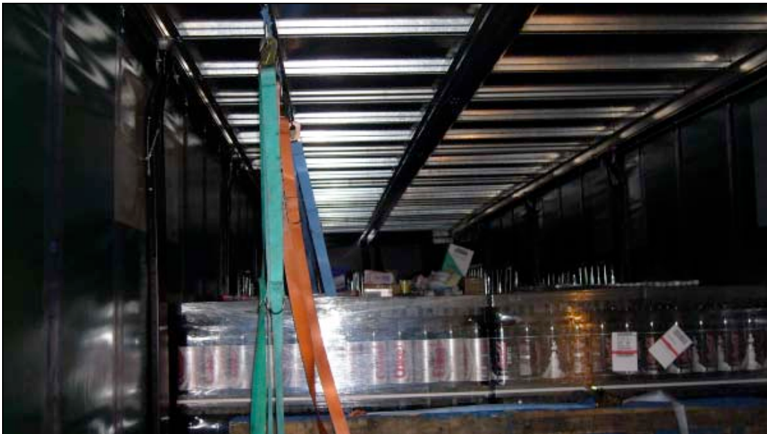
Roof mounted rail on the haulier's trailer
