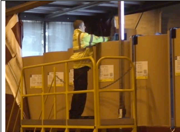
Photograph 1: The gantry allows an upright posture when throwing the webbing straps across the reels
