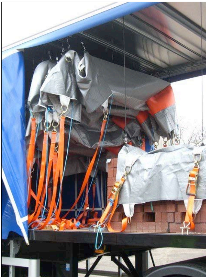
Suspended tarpaulin system used on a curtain-sided vehicle
